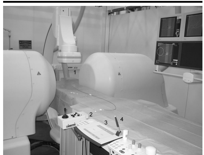
Figure 2. Photograph of the magnetic navigation system. Experimental setup with silicone liver phantom (1) and engaged magnet positioners. The tableside magnet controller (2) enables the movement of the magnet positioners. The vector tablet (3) and pen (4) are used to enter the desired orientation for the tip of the magnetic guide wire displayed on the interface screens.
